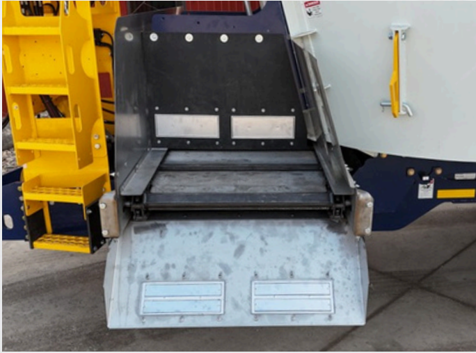
Complete Stainless Steel Conveyor Built with 1/4" Stainless Base
